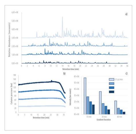
µPAC<sup>™</sup> capLC column. Based on 15 reference peptides from the Pierce<sup>™</sup> Retention time calibration (PRTC) mixture, average peak widths measured at half maximum (FWHM) between 0.10 and 0.11 min were achieved for the 30-min gradient separations at all flow rates.
