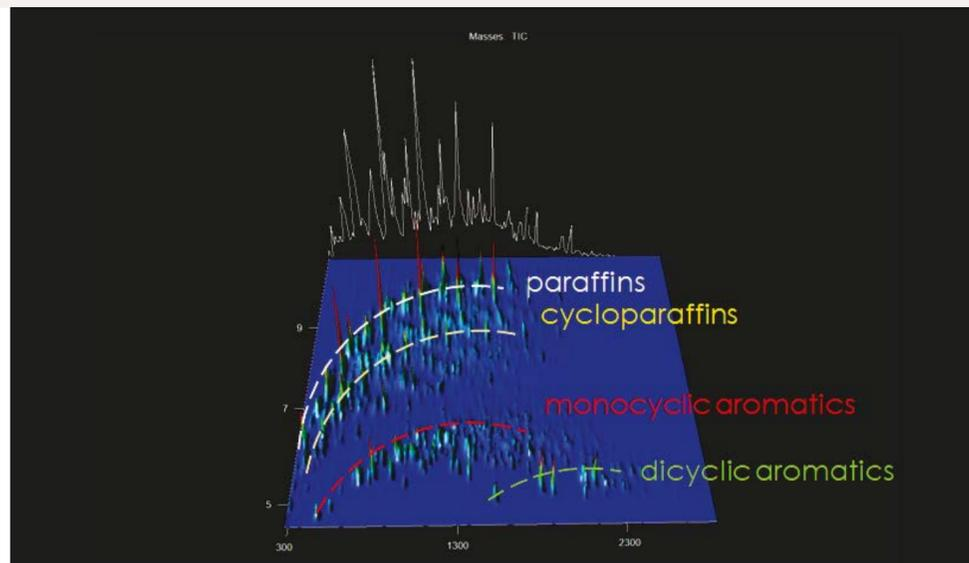
GCxGC 3D surface plot of commercial aviation turbine fuel with Total Ion Chromatogram (TIC) shown. Reconstructed trace of what a single dimension of GC separation would have looked like is shown in white. Elution bands of paraffins (white), cycloparaffins (yellow), monocyclic aromatics (red), and dicyclic aromatics (green) are indicated by dotted lines.
