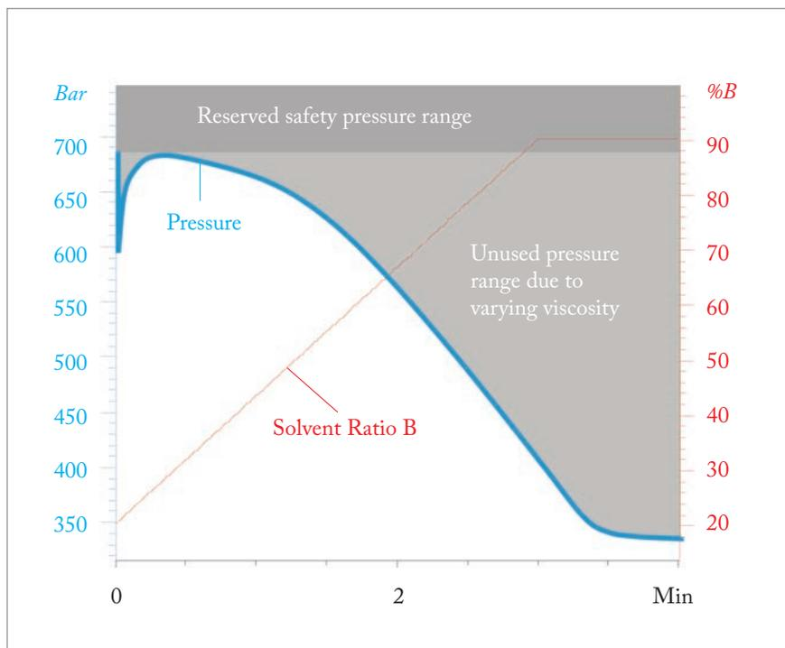
Fig 1: Typical Pressure trace for a gradient from 20 – 90 % acetonitrile
