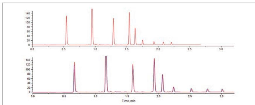
Fig 2: Separation of alkylphenones in constant pressure mode (1000 bar) (upper trace) and constant flow mode (0.6 ml/min) (lower trace, red = constant pressure vs virtual time, blue = constant flow vs real time).
