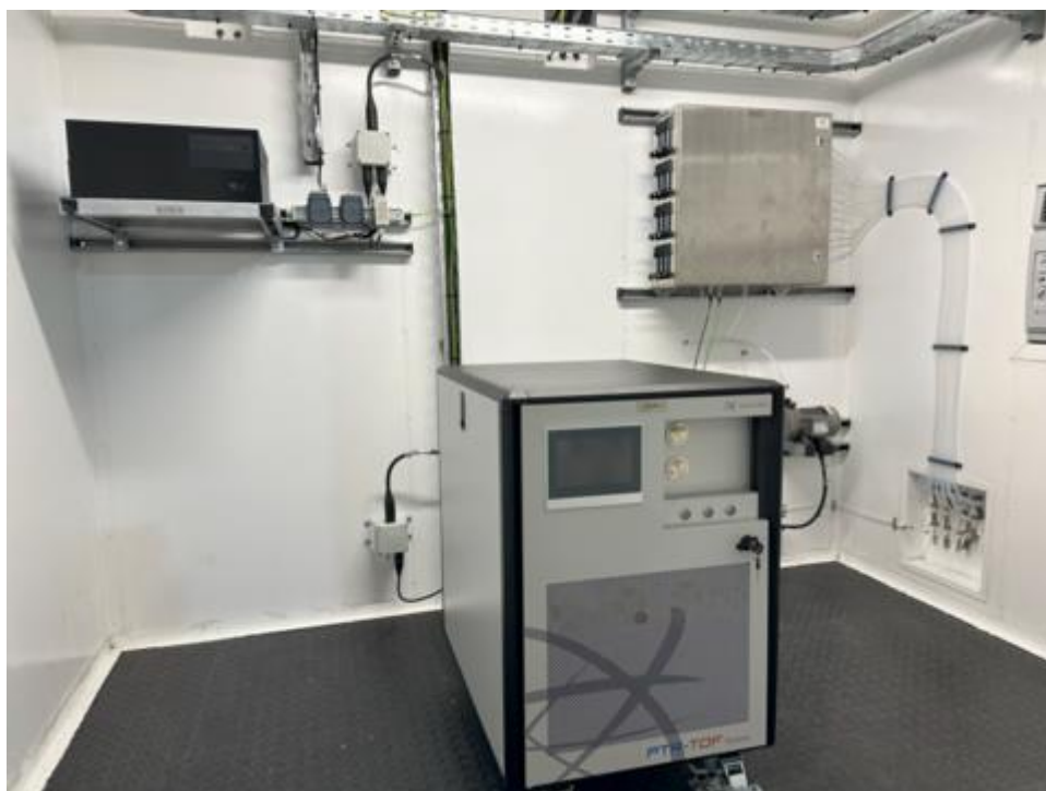
PTR-TOF real-time VOC analyzer (bottom), Sample Handling System (upper right) in the air conditioned shelter.
