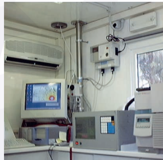
Figure 3. A mobile laboratory with a lab-made automatic chloride monomer and dichloroethane monitor, equipped with an air monitoring station and on-line diffusion model running in real time.
