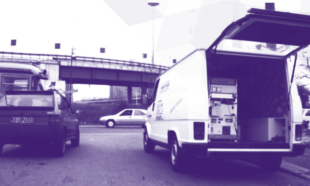
Figure 2. BTEX on-the-road monitor installed on a ZEV prototype from Fiat. Both vehicle and GC-MS instrument were powered with 12 V batteries, providing a maximum of two hours' operation time.
