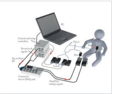
oxygen line, and one through a water-vapor line. "The latter is employed for normalization purposes, since the concentration of water vapor is determined by the temperature only, which is known," says Krite Svanberg. "The problem with unknown optical path length through the scattering medium can then be largely eliminated to yield calibrated oxygen gas levels."
