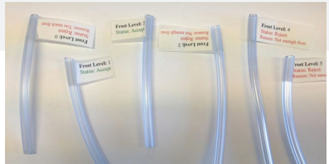
Figure 1: Although differences in the frosting levels of plastic tubing samples are difficult to distinguish visually, spectroscopic methods are highly reliable in characterizing tubing properties.
