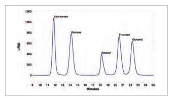
Figure 1: Chromatogram of baseline separated compounds in a standard solution of 75 mg/ml
