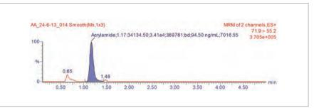
Figure 1: Chromatogram of untreated potato chip (crisp) extract showing level of incurred acrylamide.
