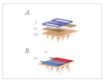
Figure 4. Illustration shows before (A) and after (B) stages of assembly of an example microneedle array platform. A: (i) microneedles, (ii) polycarbonate membrane and (iii) drug reservoir. B: assembled drug delivery system; (iv) and (v) are the drug reservoirs.
