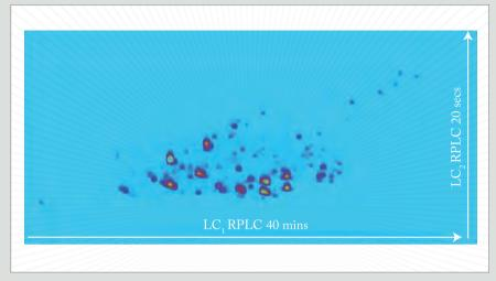
Figure 1. RPLC x RPLC 2D plot of polyphenols in green citrus tea recorded by UV at 320 nm. The first column is a C18 with a mobile phase gradient from 0.1% formic acid in water to methanol. The second column is a Phenyl-Hexyl with a mobile phase gradient from 0.1% formic acid in water to acetonitrile.
