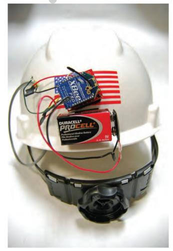
Integration of gas sensor technology into a worker's helmet by Virginia Tech researchers enables carbon monoxide monitoring.
