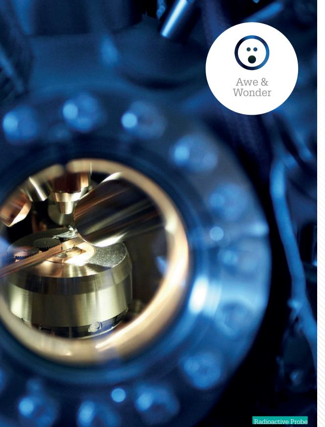
Investigating the chemistry of the inner surface of nuclear fuel cladding for radioactive materials with an X-ray Photoelectron Spectrometer. Photo credit: Canadian Nuclear Lab
